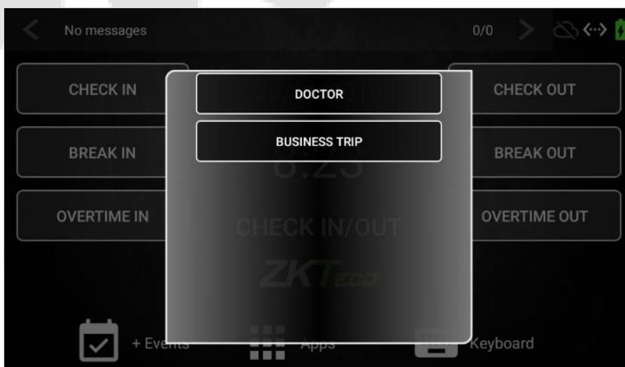
2. Make the attendance punch on the device by Fingerprint or Card. If you want to register the attendance through Password, press the Keypad on the screen and type the password.
