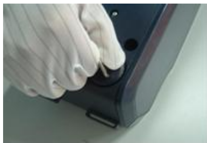
Fig. 6-5 Unscrew the air filter cap
