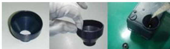
Fig. 6-7 Fill the sieve material with the funnel
