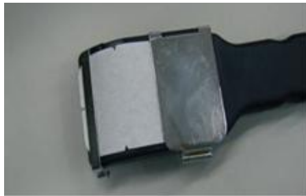
Fig. 5-9 Wipe sampling unit with paper
