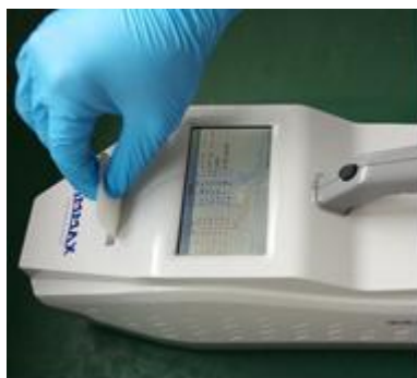
Fig. 5-18 Insert the sampling paper to the slot
